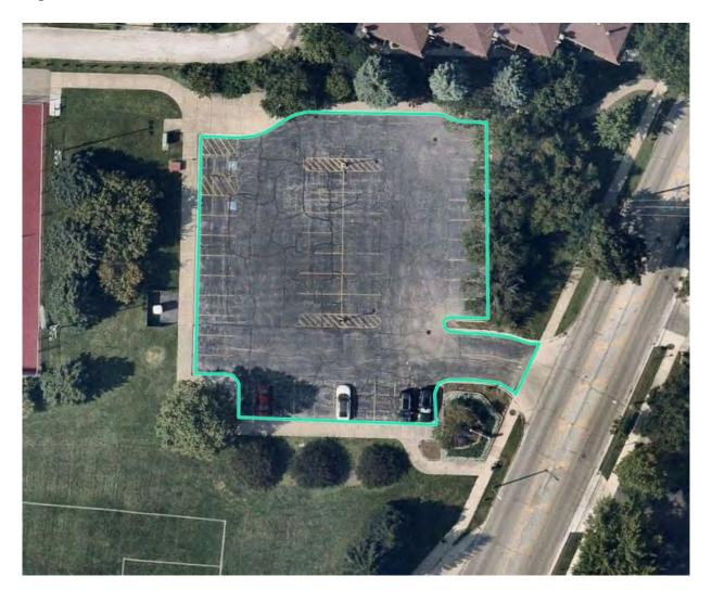
**Scope:** The scope of this project is a 2"mill and pave of the parking lot. Bidder is also responsible for repainting the parking lot lines, matching the existing layout.
