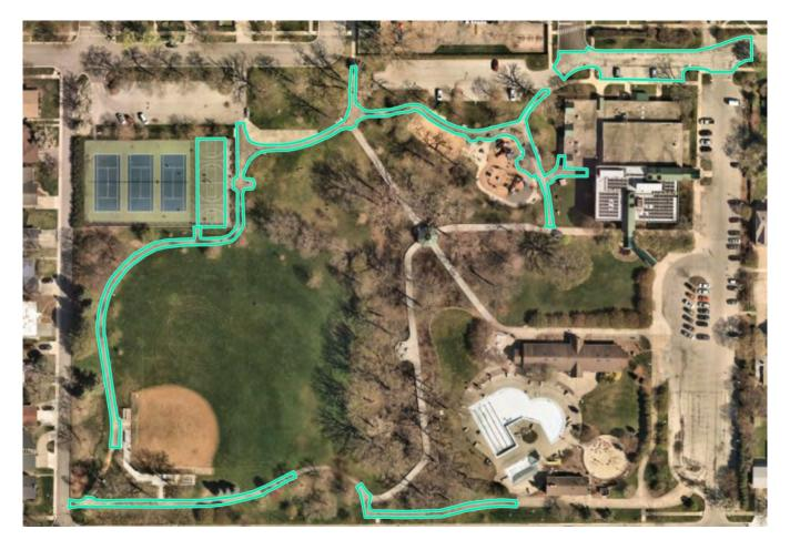
**Scope:** The scope of work at this site is a 2" milling and paving of the pathway system as shown in the overhead above, north parking lot section and basketball court. Bidder is responsible for coordinating a fence opening at the basketball court to provide access for equipment. The approximate area to be milled and paved for all areas combined is approximately 32,900 sq/ft.
